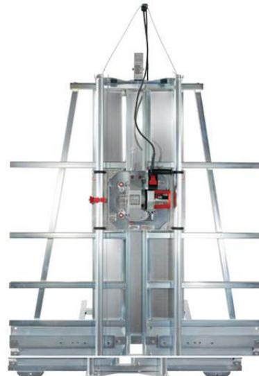
2. When cross cutting (cutting against the grain of the wood) let the saw blade come to a full stop before raising it up for the next cut. When cross cutting cut from the top only.
